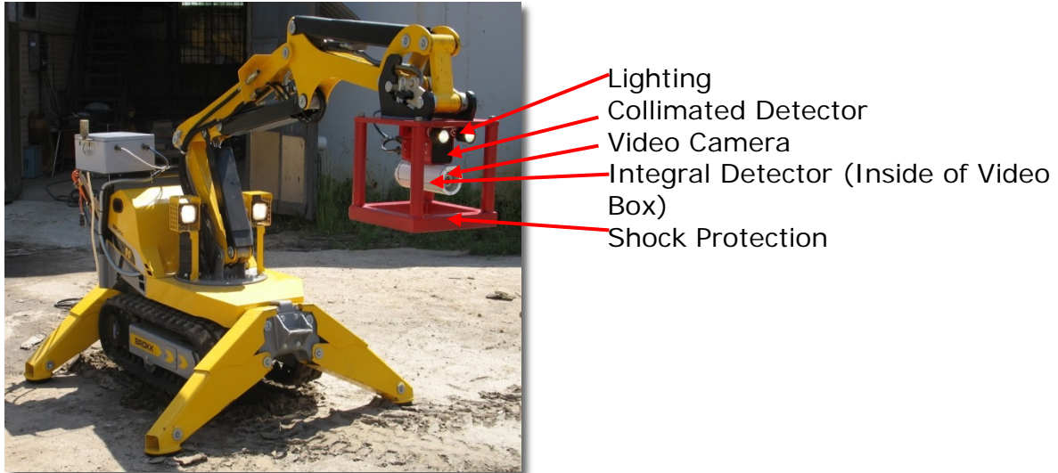
Fig. 2. System G_P installed on arm manipulator of robot Brokk.
