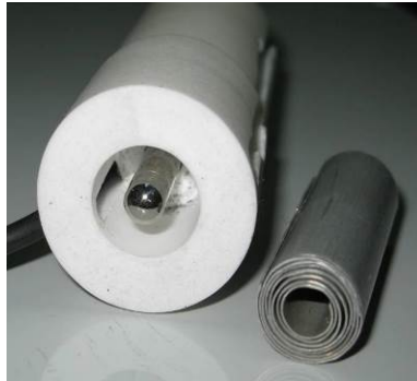
Fig. 7. Detectors of G_L : CdZnTe detector
