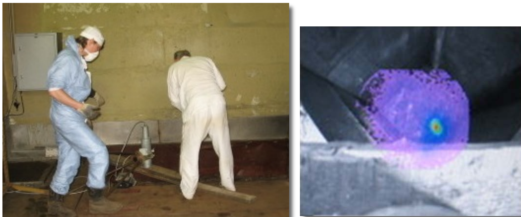
Fig. 12. Test with G_V of residual contamination of radwaste storage after discharge - left. Gamma-ray image shows presence of small lost source on bottom - right.
