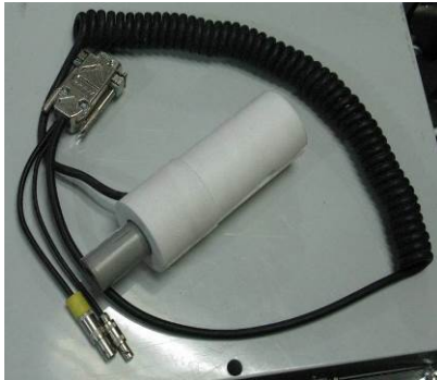
Fig. 7. Detectors of G_L : CdZnTe detector
